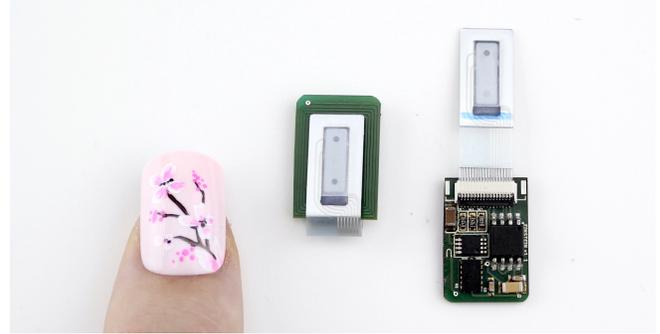
Figure 1. TransformationNail is a small fingernail worn device that attaches to the nail with acrylic nail glue. The core component is a custom designed PCB (right) that includes an e-ink display, among other components. The e-ink display folds over to make the nail more compact (middle). The size of the nail is comparable to a generic acrylic nail (left).
