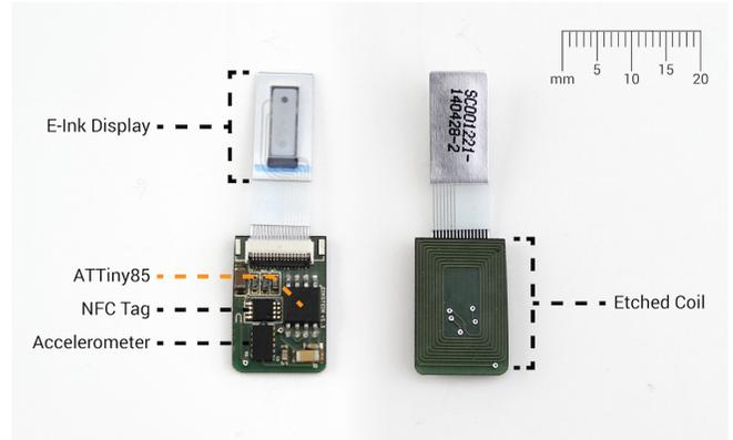
**Figure 2.** Custom designed PCB containing an e-ink display, ATTiny85 microcontroller, NT3H1101 NFC tag, and an ADXL345 accelerometer. A coil is etched into the backside of the board for both data and power transfer. The size of the PCB is 13.45mm x 19.85mm and 3.55mm thick.
